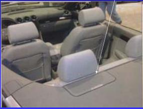
The image shows the interior of a car with the active rollover protection system (rollbars) deployed. A red arrow points to the rollbars with the text "DO NOT COVER".
