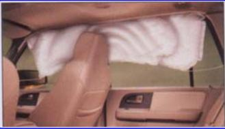
Currently, it is safe to physically cut the roof airbag open and move or remove it from the patient work area.
